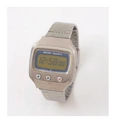
Size (dimensions of movement with LCD panel): (W)26 x (D)29.2 x (H)8.35 mm Accuracy: ±10 sec/month, avg. Display: Field-effect liquid crystal Case material: Titanium
