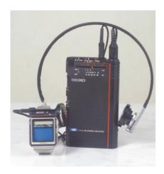
Power consumption: Approximately 520 mW with the television on
