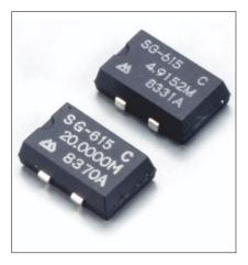
Oscillator with built-in AT-cut crystal unit sealed in heat-resistant cylinder Reference output frequency range: 1.0250 MHz - 26.00000 MHz Output enable function included Operating voltage:  $5.0 V \pm 0.5 V$ Operating temperature:  $-40^{\circ}$ C to  $+85^{\circ}$ C Soldering conditions:  $\leq 260^{\circ}$ C x 10 sec. Max. x 2 times or less; or  $\leq 230^{\circ}$ C x 3 min. or less Dimensions: (W) 14.00 x (D) 8.65 x (H) 4.7 mm Current consumption: 25 mA MAX.
