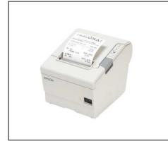
Printing method: Line thermal Print speed: 300 mm/sec max. Fonts:  $12 \times 24 / 9 \times 17$  (ANK),  $24 \times 24$  (kanji) Character size (W x H):  $1.41 \times 3.39$  mm /  $0.99 \times 2.40$  mm (ANK),  $3.39 \times 3.39$  (kanji) Print density: 180 dpi x 180 dpi Paper size\*: Thermal roll paper 79.5  $\pm 0.5$ (W) x 83 mm dia. Characters per line\*: 42/56 (ANK), 21 (kanji) External dimensions (W x D x H):  $145 \times 195 \times 148$  mm Weight: Approx. 1.6 kg (printer body)
