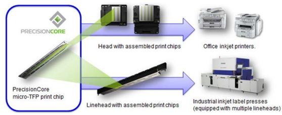
PrecisionCore are the core devices in a wide range of Epson printer products
