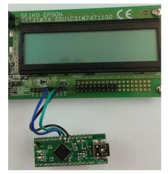
Figure 2.2.2.1 USB UART Board Connection to S5U1C31W74T1 Evaluation Board
