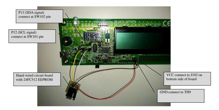
Figure 2.2.3.1 I2C Serial EEPROM Connection to S5U1C31W74T1 Evaluation Board
