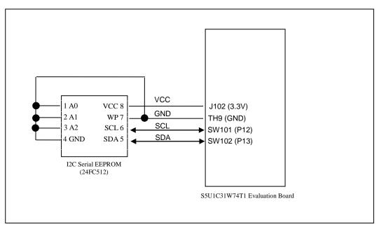
Figure 2.2.3.2 I2C Serial EEPROM Wiring to S5U1C31W74T1 Evaluation Board
