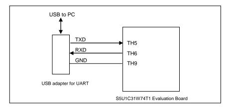
Figure 2.2.1.4 USB UART Board Wiring to S5U1C31W74T1 Evaluation Board
